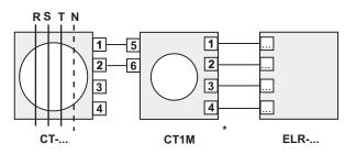
**CT1M:** It's a multiplier for the current setting of those ELR's up to 250 A. It's placed between the ELR and the measuring T/T (It isn't a wire passing through transformer)
